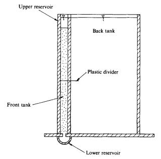
FIGURE 1. Cross-sectional view of the apparatus. Not to scale.
